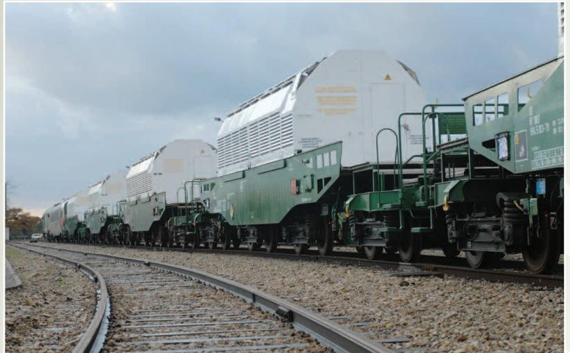
tons for truck transport and between 75 and 125 tons for rail shipments, including the weight of the used fuel. Typically, for every ton of used fuel, there is about 4 tons of protective shielding. The containers can withstand high-speed crashes, long-lasting fires and submersion in water, all without breaking open.
